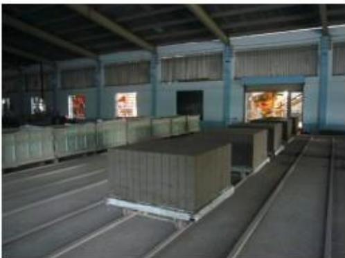
*Mobile mold trays with bricks after cut 96 bricks 7.5x 20 x 60cm are cut nicely*
